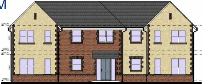
PROPOSED FRONT ELEVATION SCALE @ 1:100
