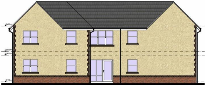
PROPOSED REAR ELEVATION SCALE @ 1:100
